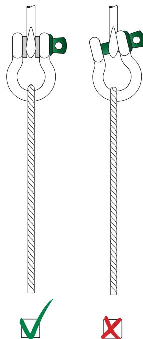
When a shackle is used to connect two slings to the hook of a lifting device, a bow type shackle must be used. The slings must be connected to the shackle body, and the shackle pin must be placed in the hook. The angle between the slings should not exceed 120°. If symmetrically loaded the shackle may be used to the full WLL.
